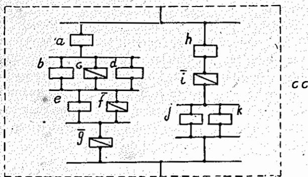
$$\{[a \cdot (b \vee \bar{c} \vee d) \cdot (e \vee \bar{f}) \cdot \bar{g}] \vee [h \cdot \bar{i} \cdot (j \vee k)]\} \therefore X$$
